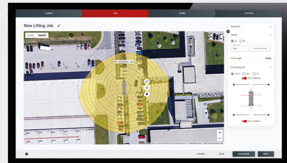
Simulate the working radius and stabilizer pressure depending on stabilizer position and load.
