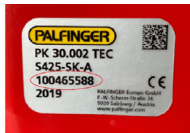
Example of equipment no.
