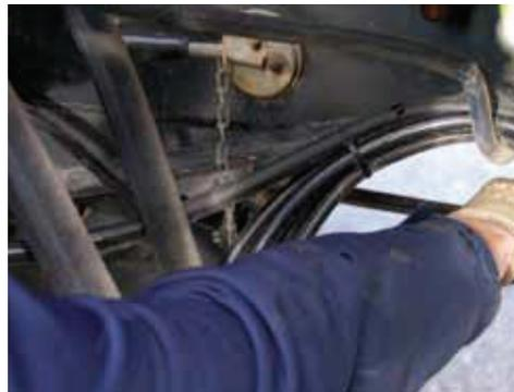
Release holding clip and clamping claw
